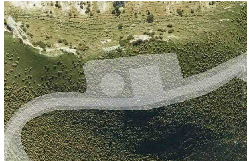
Fig. 47 Tussock grassland with 8m cuts into Amuri dip slope at turbine A18.
